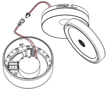
[4] Connect the plug and coupling of the secondary side.
