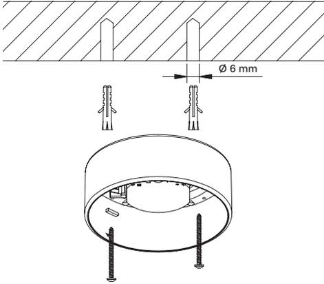
[1] Mount the housing base on a level and solid foundation. Adjust the included mounting material if necessary for different surfaces.
