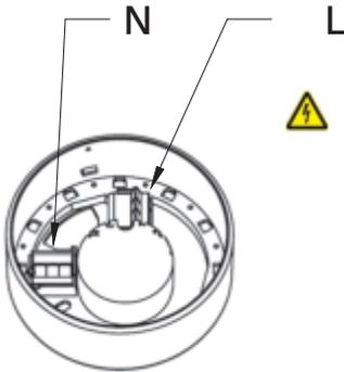
[3] Create a 230 V connection, observing occupational safety. The clamps can be unlocked with the brackets. Operation only with locked brackets.
