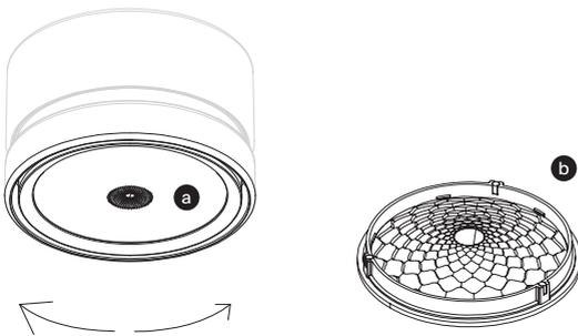
[7] The lens insert (a) is held in the luminaire by three magnets; with a slight rotation of the lens insert in the luminaire (b), the magnets separate, and the lens insert (b) falls out.
