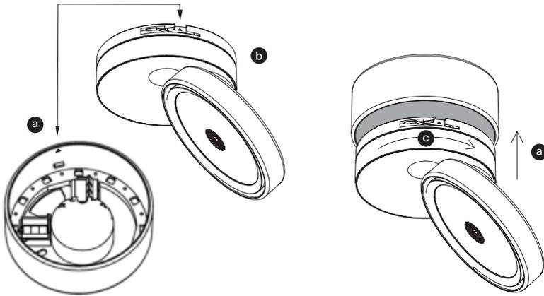
[5] Insert the insert (b) into the fit of the housing base (a), press it down, and rotate it about 20° to the click with a right turn (c). The correct position is marked with arrows.
