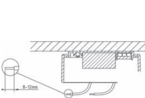
[3] Disconnect the circuit, observe occupational safety! Shorten the 230V AC cable and remove 8 mm of insulation from the conductor ends of L and N.
