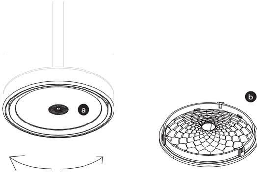
[8] The lens insert (a) is held in the luminaire by three magnets; with a slight rotation of the lens insert in the luminaire (b), the magnets separate, and the lens insert (b) falls out.
