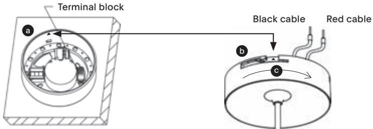
[5] Connect the red and blue wires of the luminaire housing to the terminals of the base. Observe polarity: red to + and blue to -
