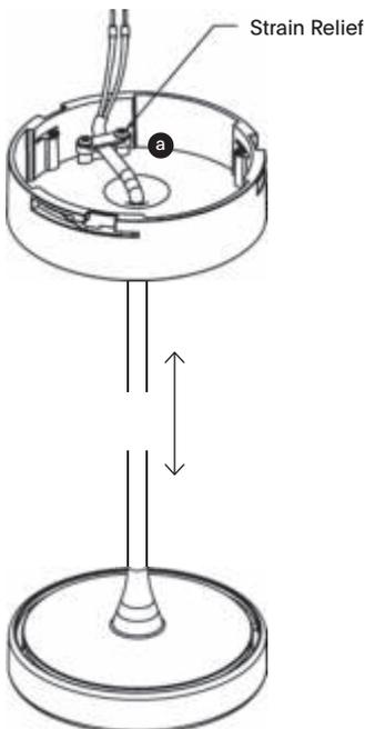
[8] Loosen the screws of the strain relief (a) and set the cable to the desired pendant length. Strip the conductor ends and crimp them with the included end sleeves.
