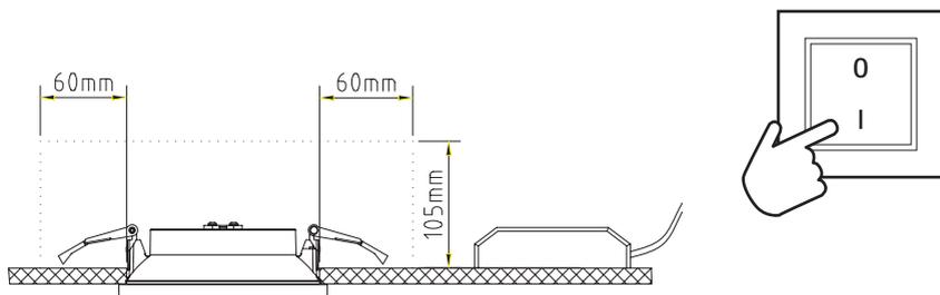
[5] Please observe the recommended minimum distances in the ceiling for cooling the luminaire. Do not cover the luminaire and driver with insulating material.
