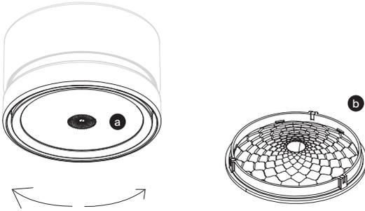
[8] The lens insert (a) is held in the luminaire by three magnets; with a slight rotation of the lens insert in the luminaire (b), the magnets separate, and the lens insert (b) falls out.
