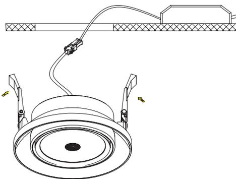
[3] Connect the driver and the lamp with the connectors.
