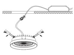
[4] Push both spring clips upwards and place the downlight into the ceiling.
